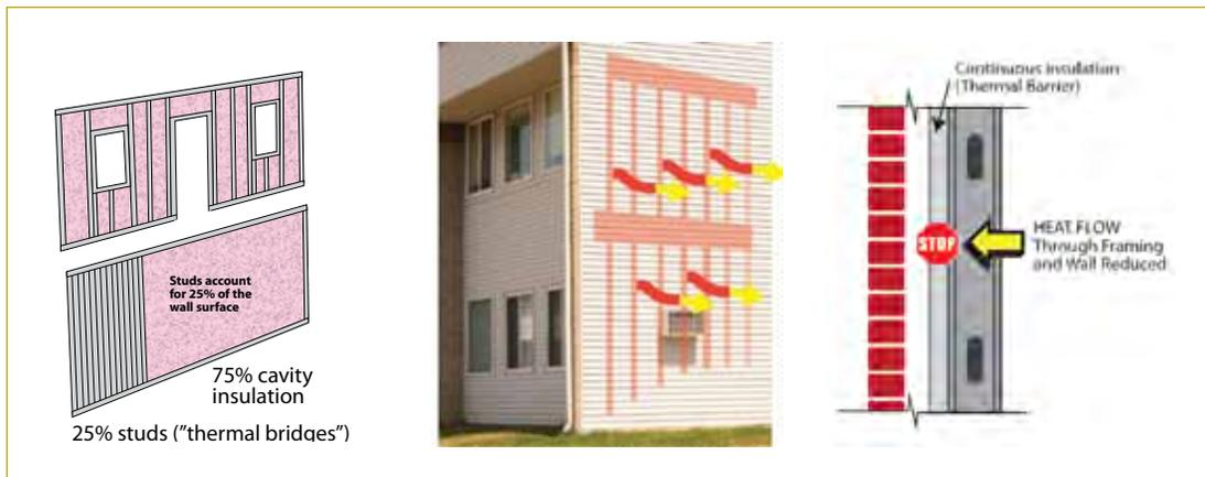
Figure 2. Thermal bridging through wall framing causes a disproportionate amount of heat loss. With continuous insulation, heat loss from thermal bridging is minimized providing a favorable economic and environmental benefit over use of cavity insulation alone.
