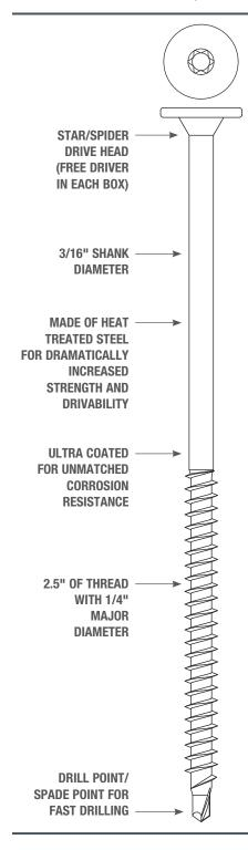
Hunter Panels SIP SD Fastener is intended to mechanically attach Hunter Xci NB, Hunter Xci Ply or Xci Ply (Class A) to CMU, Concrete or Steel Stud wall types. Hunter Panels SIP SD Fastener has the following features:
